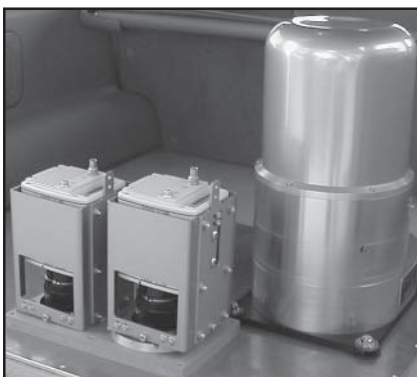
FIGURE 1: This is a photograph of the Firemapper(tm) airborne system. The system consists of two visible/near-infrared digital cameras and an infrared microbolometer sensor.
