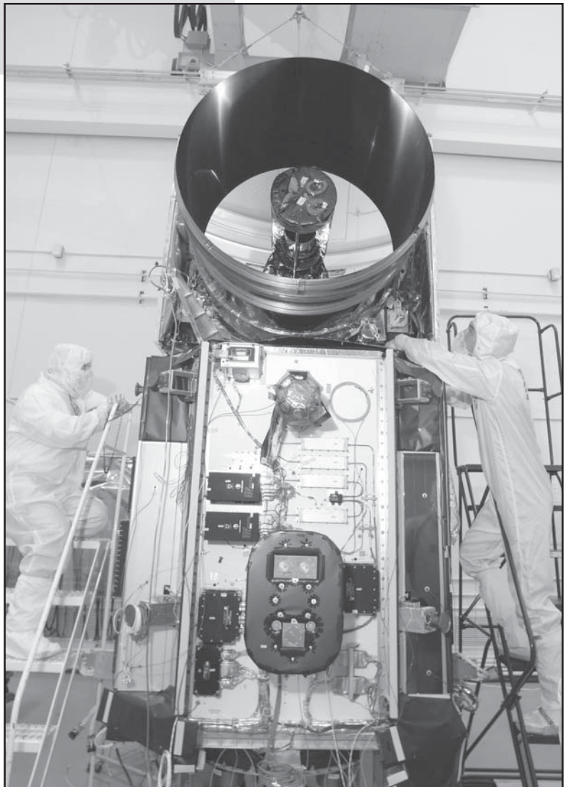
FIGURE 1: The Geoscience Laser Altimeter System (GLAS) on the Ice, Clouds, and land Elevation Satellite (ICESat) spacecraft immediately following its initial mechanical integration on June 18, 2002. Note that ICESat’s solar arrays have not yet been attached. Left – Gordon Casto, NASA/GSFC. Right – John Bishop, Mantech. Photo Credit: Courtesy of Ball Aerospace & Technologies Corp.
