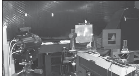
FIGURE 3 shows the experimental configuration for the lamp setup, with (left to right) the VXR, a beam block for ambient measurements, the plaque (covered by an alignment target), a lamp baffle, and the lamp alignment jig.
