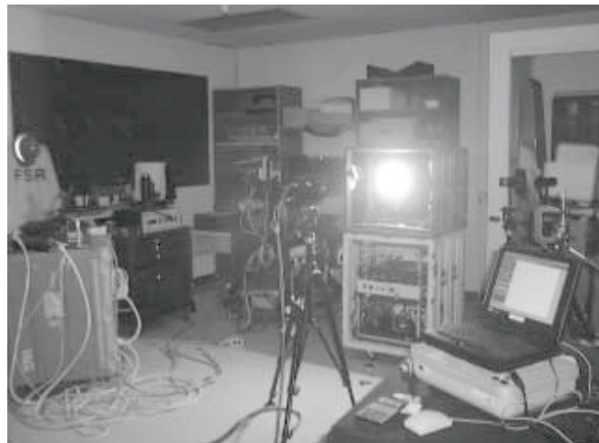
Figure 1. The NIST VXR measuring the NPR integrating sphere source at NASA Ames Research Center.
