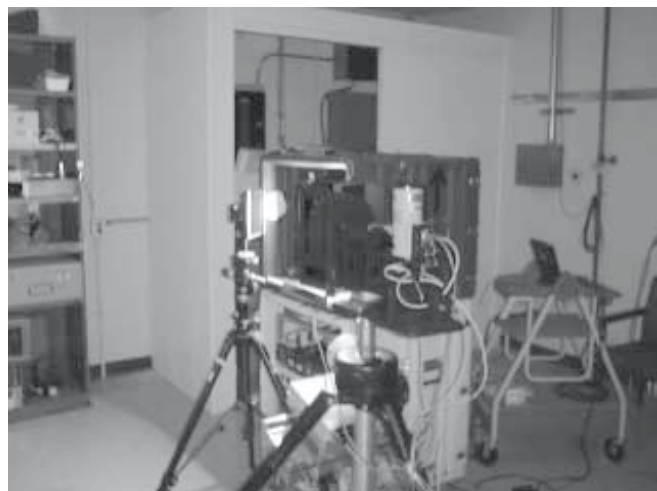
Figure 2. The UA SWIR radiometer measuring the NPR source using the fold mirror.
