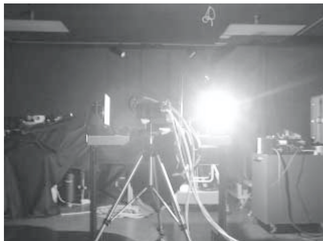
Figure 3. The UA VNIR radiometer measuring the Ames reflectance panel illuminated by a 1000 W FEL irradiance standard lamp. The radiometer is in the foreground with the white reflectance panel on the left and the bright lamp on the right.
