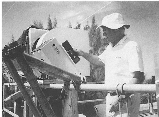
MODIS Science Team member Ian Barton (CSIRO) mounts an IR radiometer on the rooftop instrument platform.
