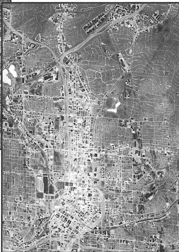
Figure 2 (bottom right) ATLAS nighttime thermal image (channel 13— 9.60-10.2 \mu\text{m} ) of the Atlanta central business district area. These data have not been geometrically or atmospherically corrected.
