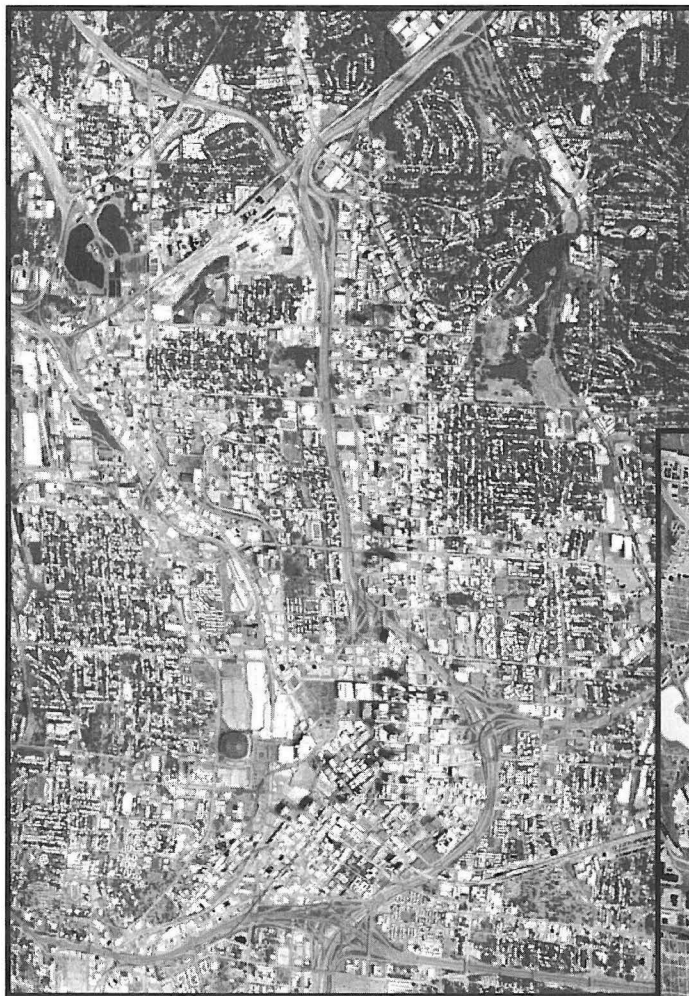
Figure 1 (top left) ATLAS daytime thermal image (channel 13— 9.60-10.2 \mu\text{m} ) of the Atlanta central business district area. These data have not been geometrically or atmospherically corrected.
