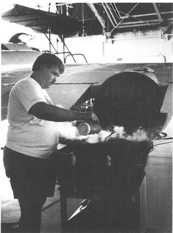
John Bush of NASA Ames pours liquid nitrogen into the dewars on the MAS (MODIS Airborne Simulator) to keep the detectors cold.
