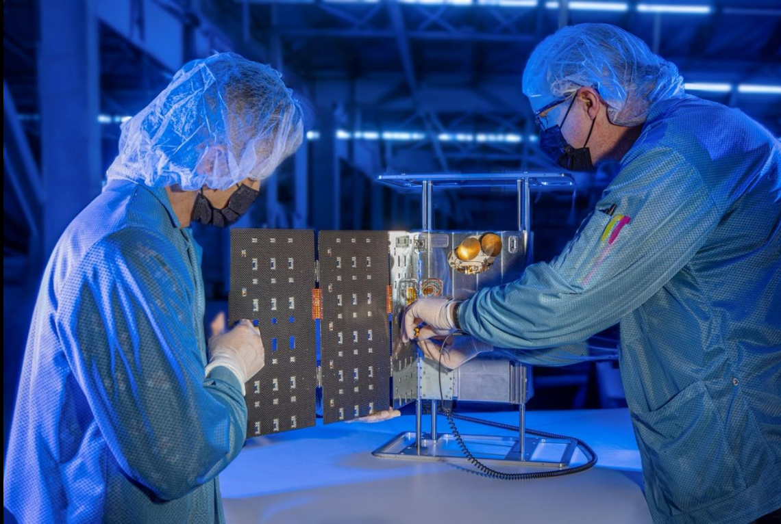
Blue Canyon Technologies (BCT) technicians Davy Hong and Dave Biancalana attach a solar array to the bus of the Electrojet Zeeman Imaging Explorer (EZIE) CubeSat. Brooks Freehill, Blue Canyon Technologies
