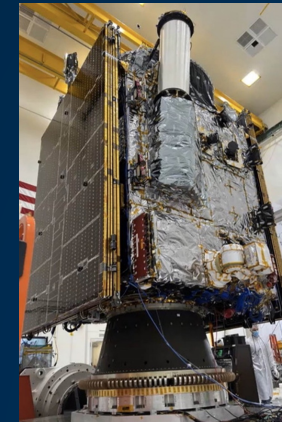
Psyche on shaker table for dynamics testing
