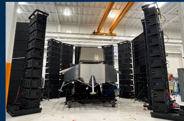
Astrobotic Griffin lander STM; acoustic testing
