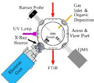
Above: ICEE UHV chamber showing radiation sources and in situ instruments.
