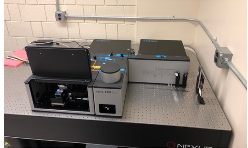
Neaspec neaSNOM near-field infrared imaging and spectroscopy system at Stony Brook University.
