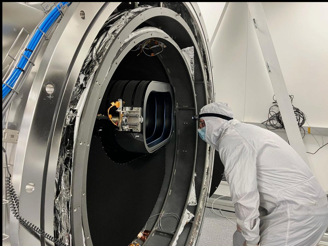
The instrument (telescope + FPAs + V-grooves) has gone through 3 cryogenic focus tests and 1 spectral calibration at Caltech. Results are excellent. All  $32 \times 6 = 192$  readout channels operate perfectly.
