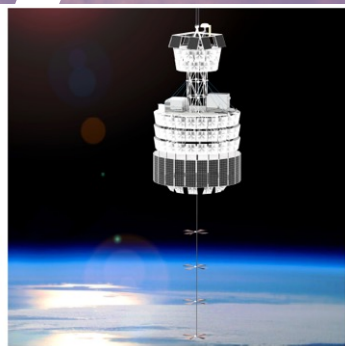
Figure 10: A rendering of the PUEO payload, including a design for the low-frequency drop-down instrument.
