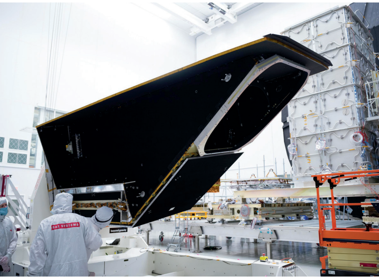
Watching Out for Too-Close Encounters of the Asteroid Kind. NASA's NEO (Near-Earth Object) Surveyor mission, seen here undergoing environmental testing in the Space Environment Simulation Laboratory at NASA's Johnson Space Center in December 2024, is the agency's first space-based detection mission specifically designed for planetary defense. Slated to launch no earlier than September 2027, NEO Surveyor's infrared detectors will seek out, measure, and characterize otherwise hard-to-find dark asteroids and comets that could pose an impact hazard to Earth. Credit: NASA/Jet Propulsion Laboratory (JPL)-Caltech
