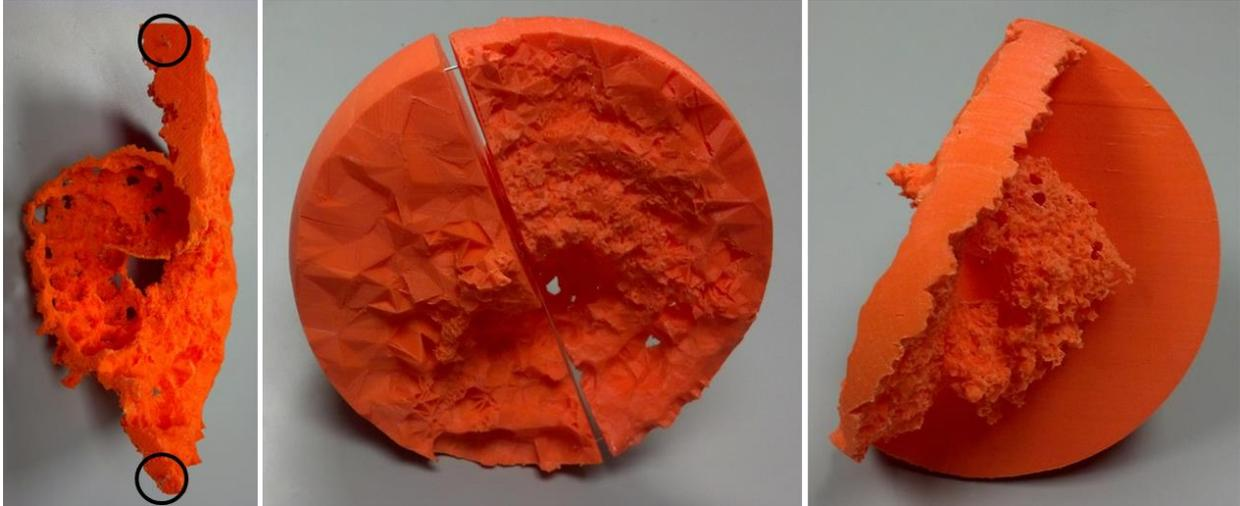
**Figure 2.** Example showing the placement of the metal pins (circled in the first panel) used to connect the two component pieces of the 3D print model at orbital phase 1.045.
