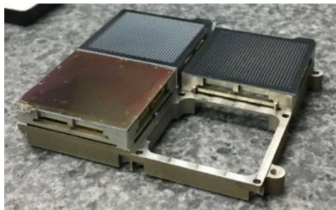
Arcus flight-like grating window w/flight-like CAT grating facet on left
