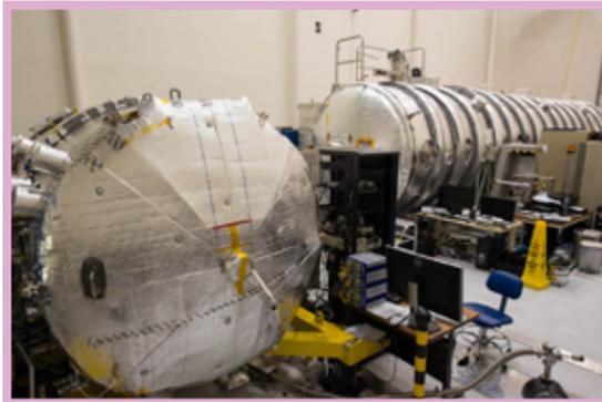
**High-Contrast Imaging Testbed (HCIT) Laboratory (JPL):** HCIT is the world's premiere facility for demonstrating and advancing space coronagraphs, hosting two vacuum testbeds and one in air, with lasers, DMs, and other optical equipment. The facility was used to demonstrate technology for the RST Coronagraph as well as SAT-funded starlight-suppression technologies that will be needed by HWO.
