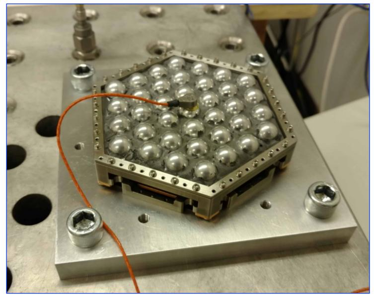
Mock array in vibration test
