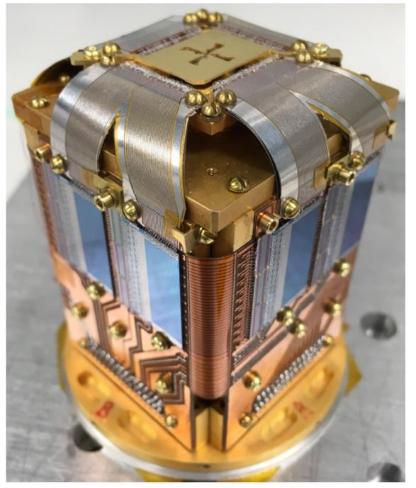
2D Delta-Doped Electron-Multiplying Charge-Coupled Device (EMCCD) detector
