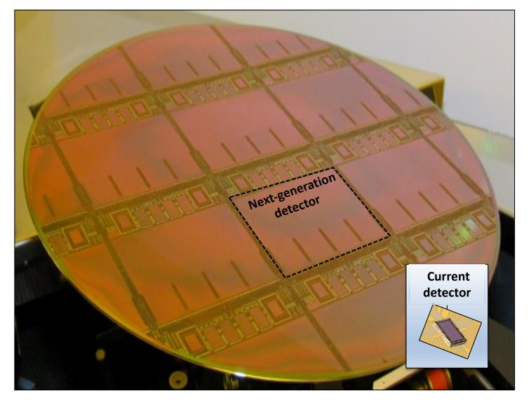
Six next-generation X-ray detectors on 200-mm wafer. Inset shows current, much smaller sensor
