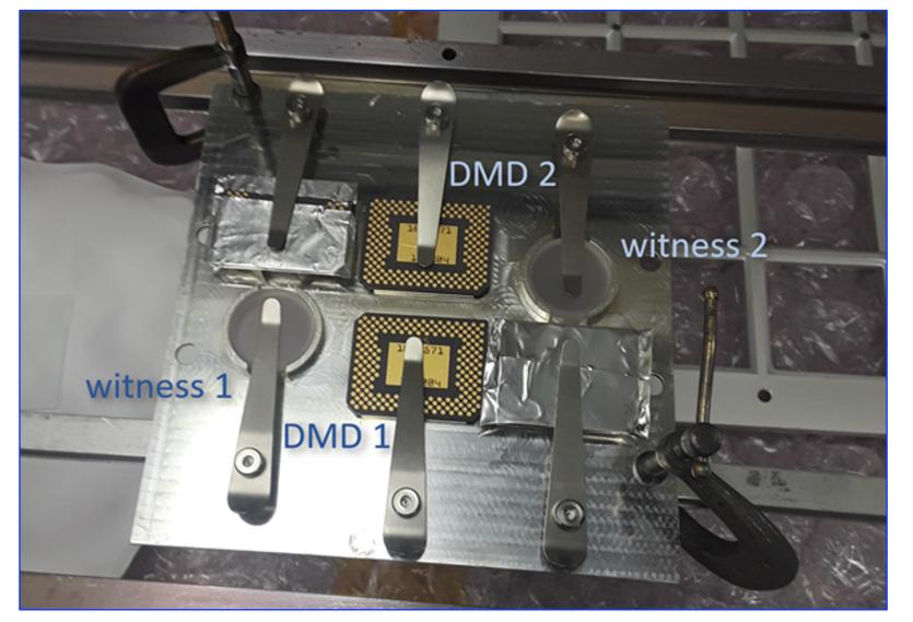
Commercially available Digital Micromirror Devices (DMDs) recoated for improved UV reflectance
