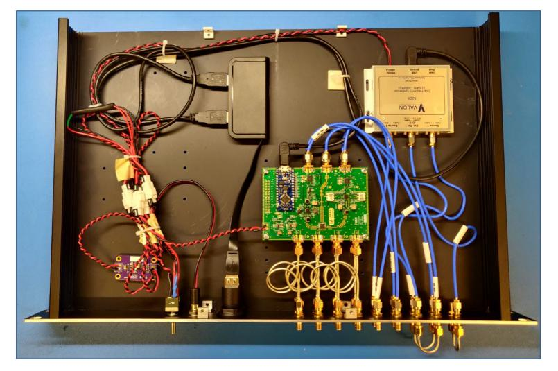
Auxiliary boards for reading out superconducting resonators with resonant frequencies from  $0.1-8\,$  GHz, implemented for ground-based Toltec experiment
