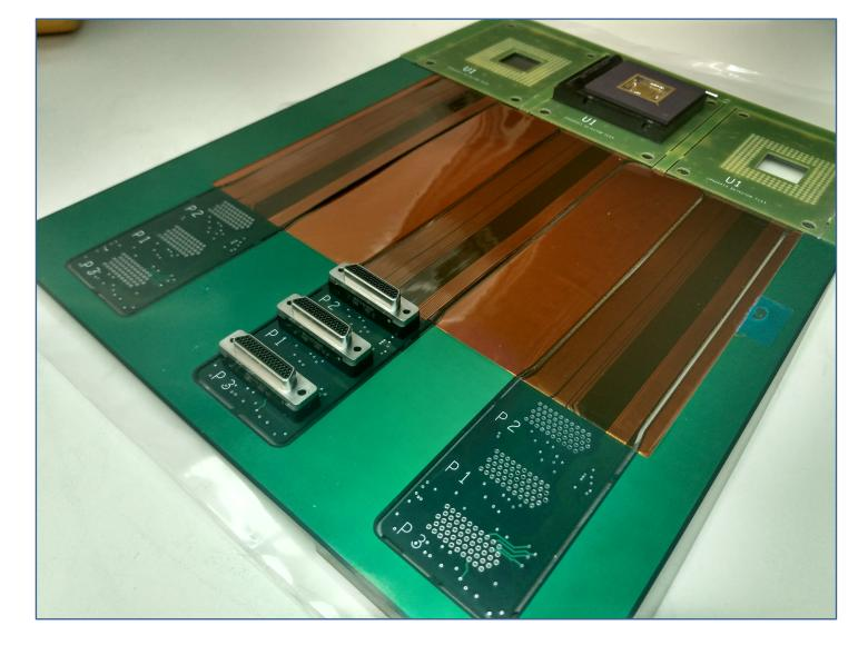
One of three assembled low-noise detector boards in a panel
