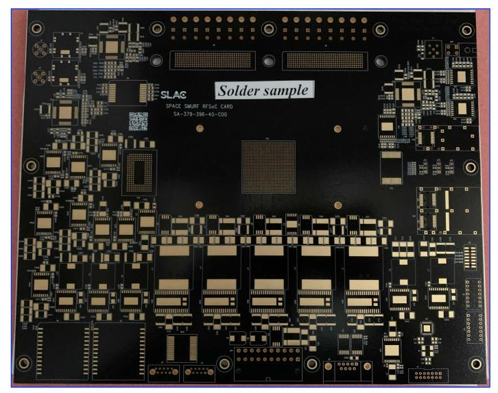
Radio Frequency System-on-Chip (RFSoC) board allowing dense readout of large focal planes
