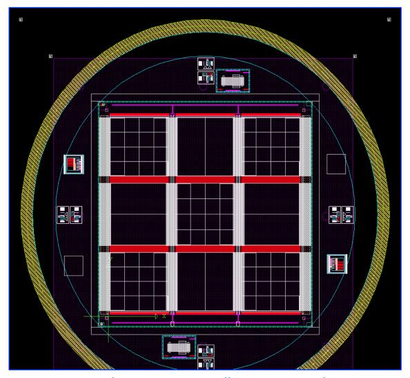
Mask layout for 734×348 microshutter array; small sections in sub-arrays consist of microshutters with various keystone structures
