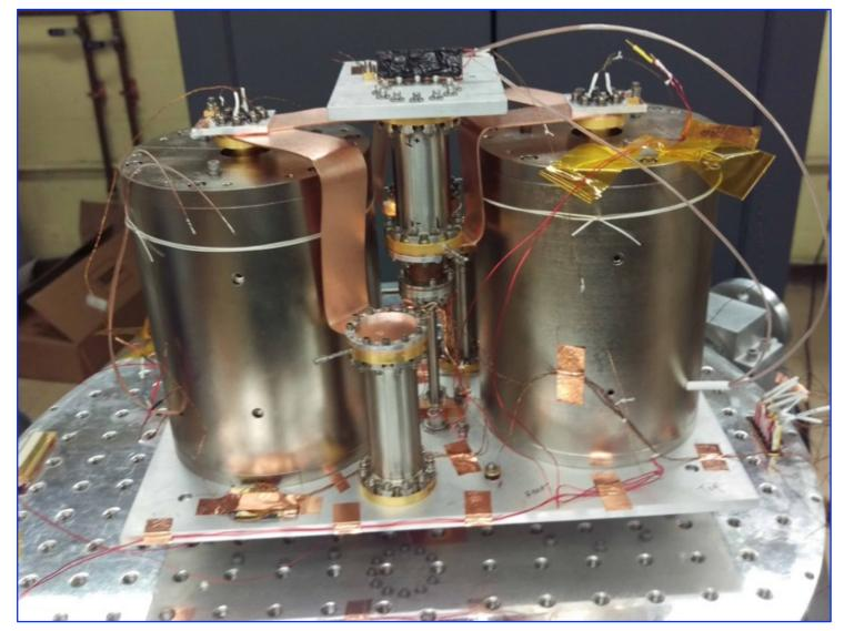
Two-stage 10K-to-4-K Continuous Adiabatic Demagnetization Refrigerator (CADR)
