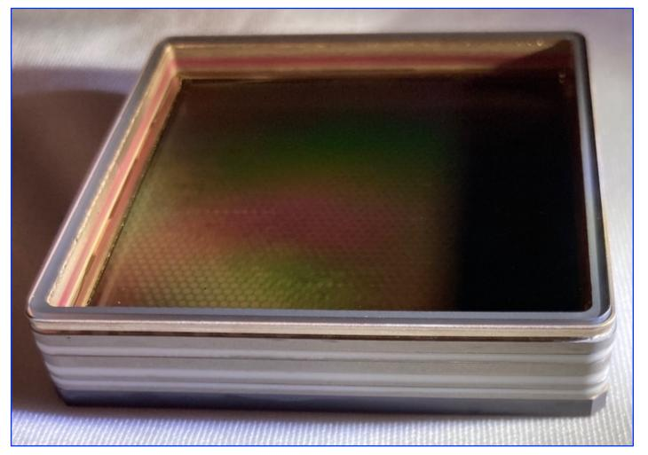
Planacon 50-mm sealed tube with sapphire input window, bialkali cathode, Atomic Layer Deposition (ALD) borosilicate Multi-Channel Plates (MCPs), and Low-Temperature Co-fired Ceramic (LTCC) XS anode
