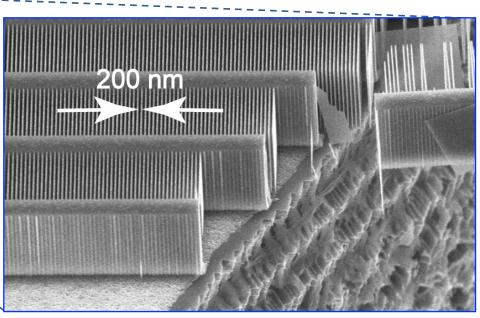
Scanning Electron Microscope (SEM) images of cleaved freestanding Critical-Angle Transmission (CAT) grating
