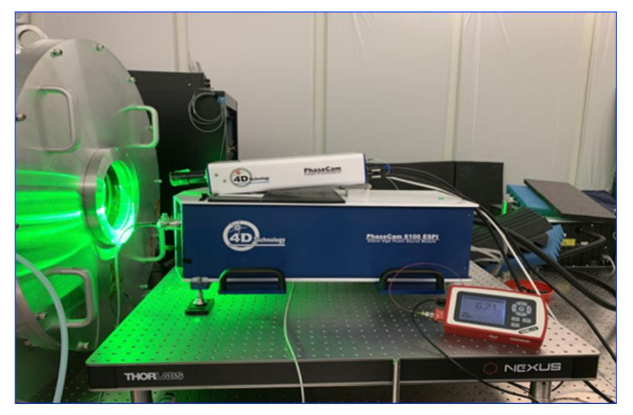
Speckle interferometer for ultra-precise measurements of non-reflective objects
