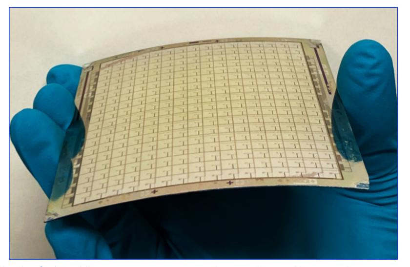
Back side of adjustable X-ray mirror segment with row-column addressing, electro-static-discharge (ESD) protection circuits, and piezo cells
