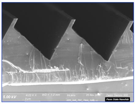
Protoflight CHESS echelle grating and Scanning Electron Microscope (SEM) image of ruled grating
