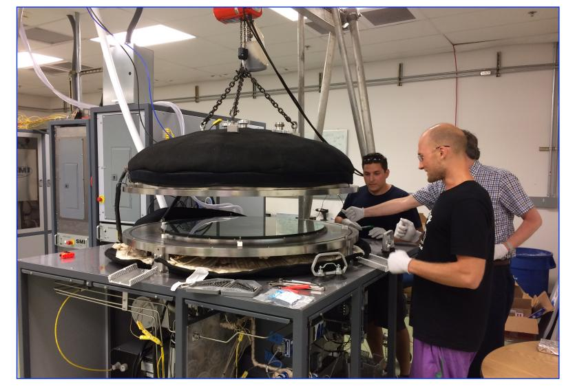
Custom 0.9-m Atomic Layer Deposition (ALD) tool, developed to coat ground-based astronomical mirrors for ALD-protected silver
