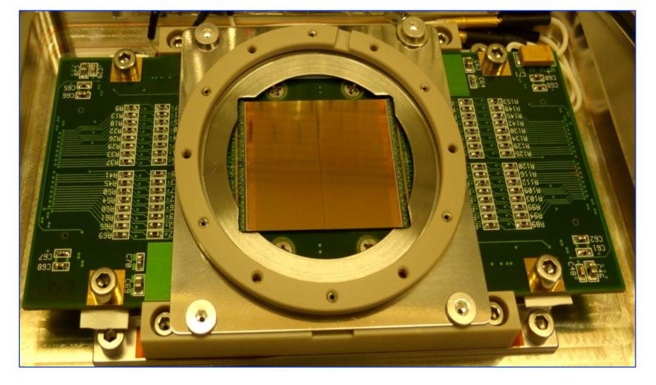
Multi-Channel Plate (MCP) detector with 2×2 array of Timepix readout chips in the center
