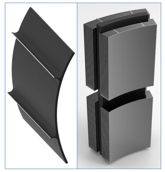
Single X-ray mirror segment with mounting ridges plus stacked segments with support panel **Significance:** World-class thin grazing-angle X-ray mirror technology; baselined for Lynx X-ray
