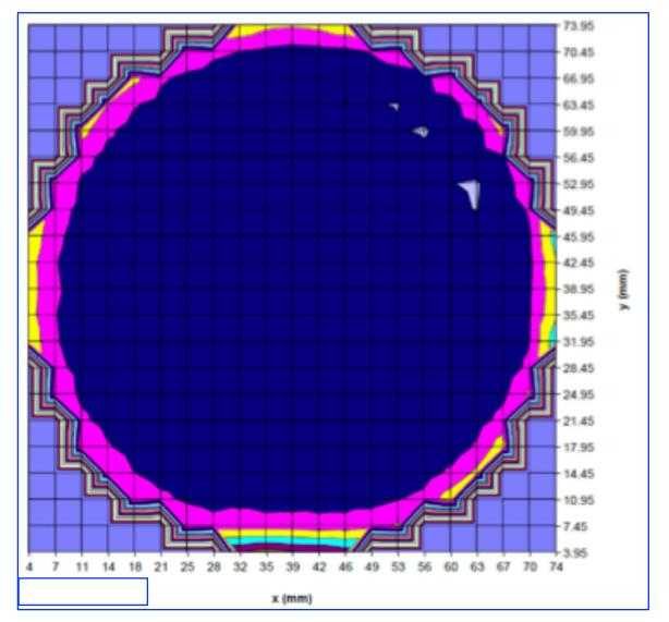
Growth uniformity of wafer yielding six usable sites for 1k×1k-pixel Linear-mode Avalanche Photodiode (LmAPD) detector
