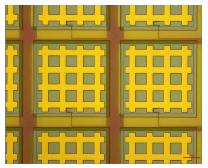
Gold:Erbium (Au:Er) "waffle" sensor targeting Lynx main array requirements
