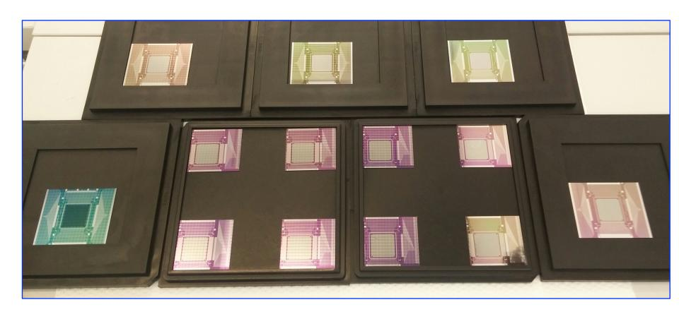
Substrates with light shields for next-generation electrostatically activated microshutter arrays
