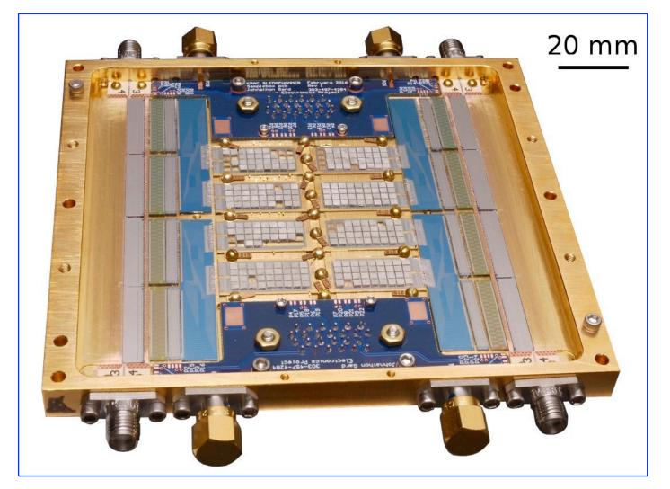
Sample electronics box with Transition Edge Sensor (TES) microcalorimeter detectors, microwave multiplexers, and support electronics
