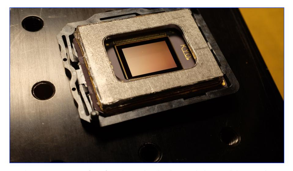
Digital Micro-mirror Device (DMD) window replaced with 2-μm-thick nitrocellulose membrane **Significance:** Replacing windows of commercially available DMDs may enable far-UV multi-object spectrometry in future missions
