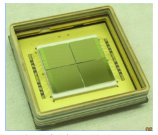
2×2 array of Timepix readout chips for Multi-Channel Plate detectors
