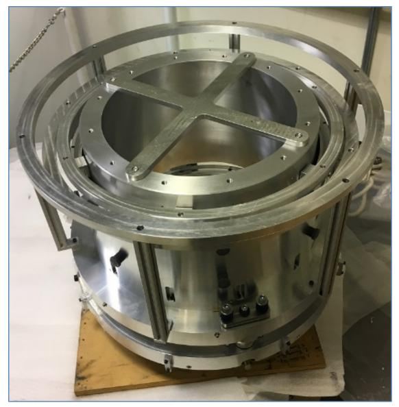
Support structure for X-ray mirror shell
