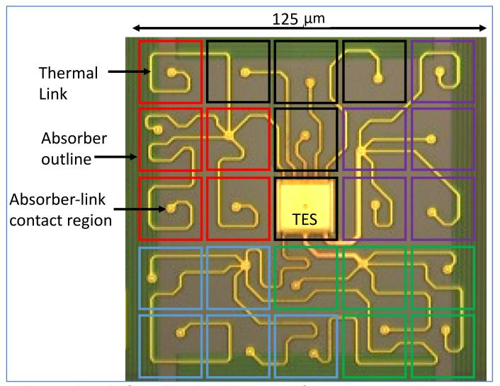
25-pixel Hydra readout before absorber deposition for X-ray microcalorimeters
