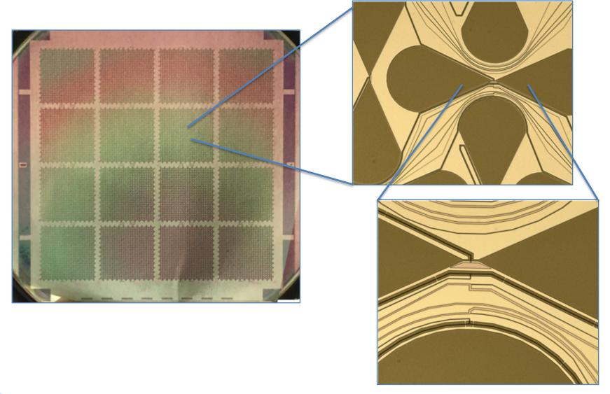
30/40-GHz bowtie planar antenna design for Cosmic Microwave Background (CMB) polarimetry
