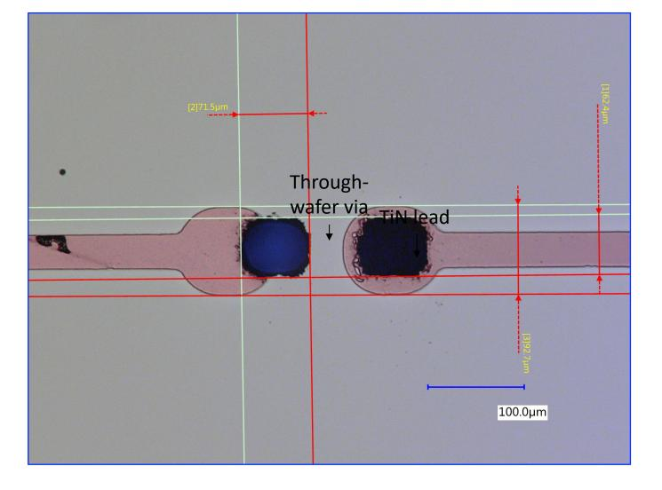
Through-wafer via allowing connection of 2D superconducting detectors to cold readout electronics
