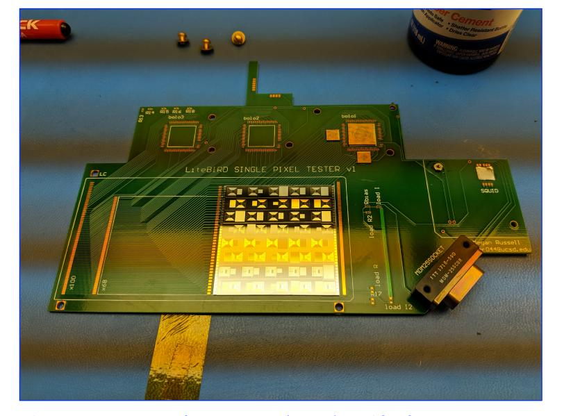
Superconducting QUantum Interference Device (SQUID) amplifier for 100-mK test
