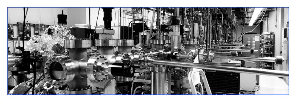
UHV system built at ASU for fluoride Plasma-Enhanced Atomic Layer Deposition (PEALD) mirror coatings
