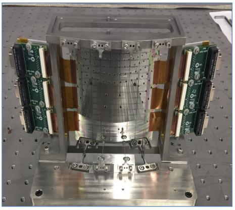
Adjustable X-ray mirror sample, with front reflective surface shown on left, and electrode control side on right
