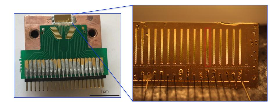
Chip carrier with printed circuit board for wiring (left), and die of 20 DFB devices indium diebonded to copper chip carrier (right)
