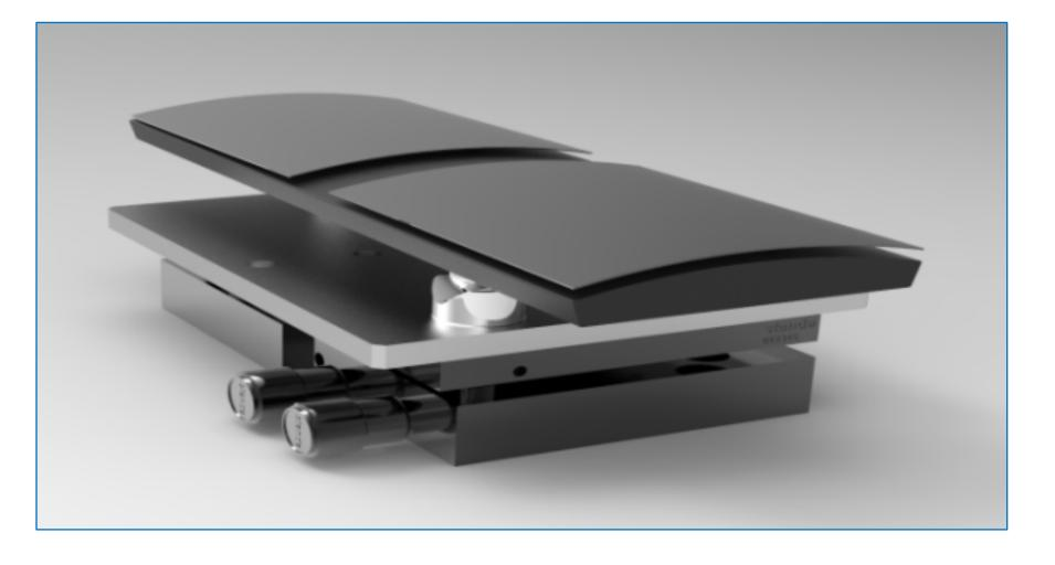
Technology Development Module with a pair of parabolic-hyperbolic X-ray mirror segments
