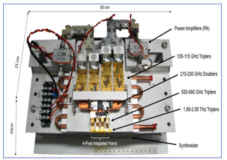
1.9-THz 4-pixel frequency-multiplied chain for Stratospheric Terahertz Observatory 2 (STO-2, launched Dec 2016)
