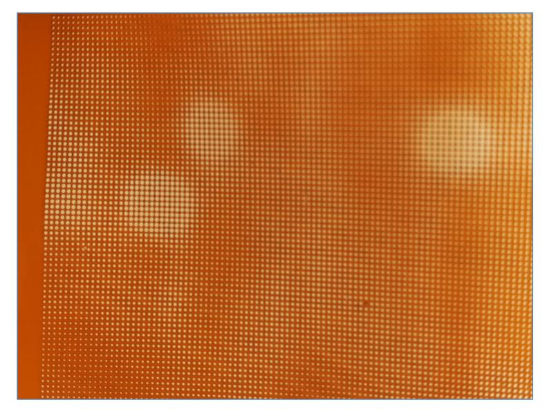
Custom coating mask with varying holes corrects entire X-ray optic in one exposure
