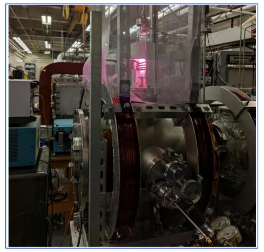
Large Area Plasma Processing System (LAPPS) reactor at NRL, used for removing oxidation from aluminum optics prior to coating
