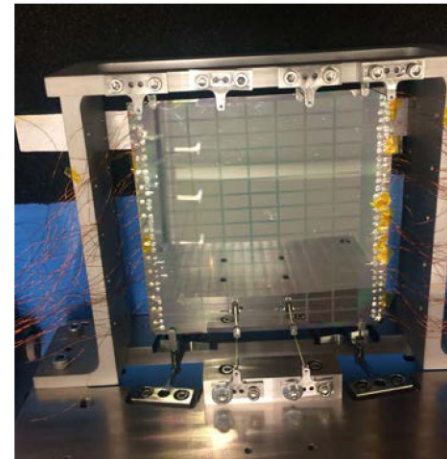
Single shell mounting concept with a mounted adjustable mirror
