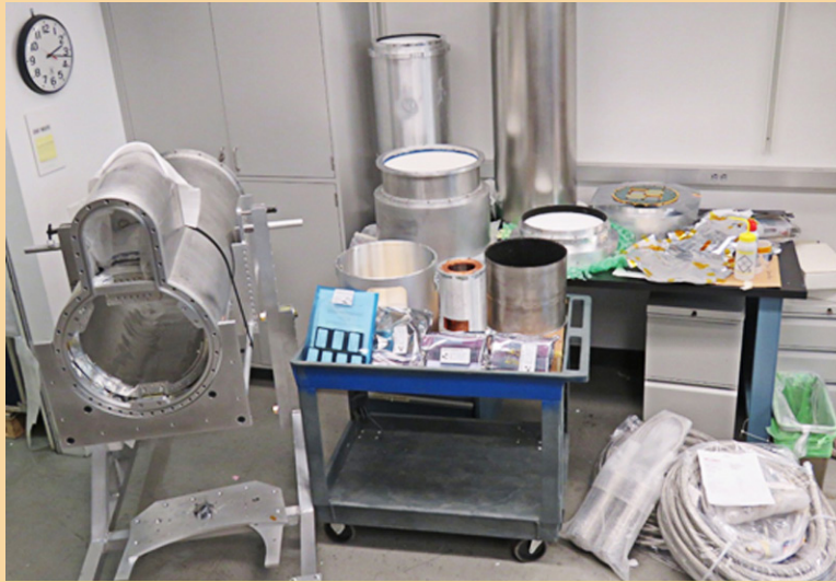
Fig. 7. Test bed for checking RF performance and carrying out future 200-350-GHz antenna development. The system is a small telescope cooled to 4 K using a pulse tube combined with a 300-mK cooler for operating the detectors.
