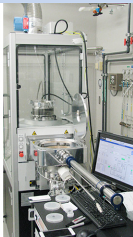
Fig. 2. Left: Calculated performance of a five-layer metal-dielectric filter on silicon or quartz substrates, showing in-band QE > 60% and out-of-band rejection approaching 10^{-4} . This is an example of detector-integrated filters that can render silicon "solar blind". Right: JPL ALD system used to deposit the metal-dielectric layers.
