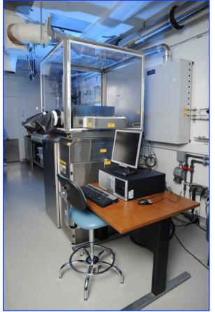
Atomic Layer Deposition (ALD) reactors at JPL used for developing advanced UV coatings
