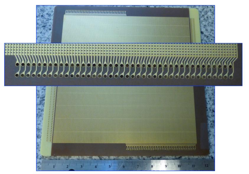
100 mm polyimide anode used for 100×100 mm<sup>2</sup> Multi-Channel Plate (MCP) detector
