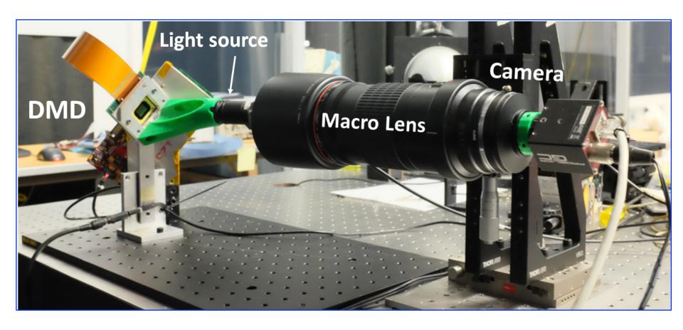
Detecting tripped micro-mirrors in Digital Micro-mirror Device (DMD) during vibration and shock testing done as part of flight qualification
