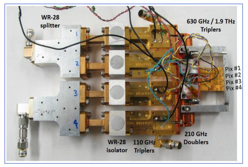
Biasless 1.9-THz triplers developed for multi-pixel Local Oscillator (LO)
