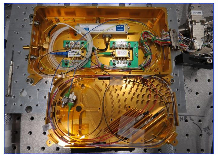
Prototype laser oscillator and pre-amplifier for lasers enabling the Laser Interferometer Space Antenna (LISA) gravitational-wave observatory
