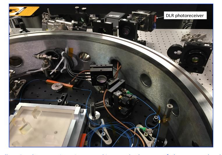
GRACE Follow-On photo-receivers integrated into testbed as part of phasemeter development for the Laser Interferometer Space Antenna (LISA) gravitational-wave (GW) observatory
