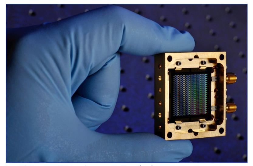
484-pixel 350-mm Kinetic Inductance Detector (KID) array
