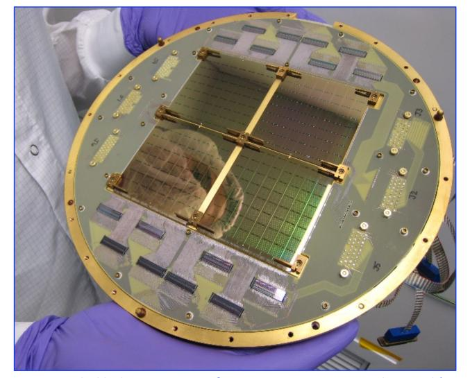
Large-format antenna-coupled bolometer arrays for Cosmic Microwave Background (CMB) polarimetry
