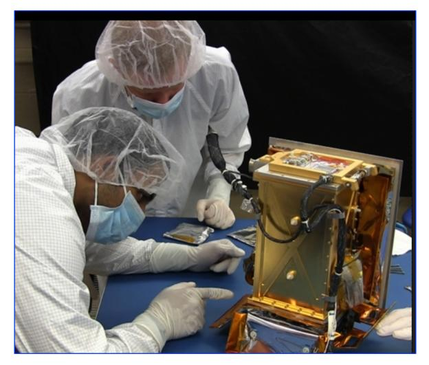
Students working on REXIS, a student-built instrument deployed on the OSIRIS-REx mission to Asteroid Bennu, that deployed with directly deposited filter on its X-ray CCDs
