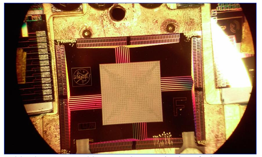
Candidate demonstration model Transition-Edge Sensors (TESs) array for the ATHENA X-ray Integral Field Unit (X-IFU)
