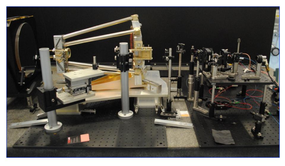
Measuring scattered light in prototype Laser Interferometer Space Antenna (LISA) telescope
