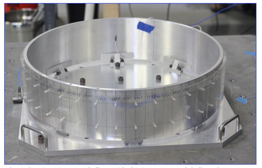
Mechanical engineering meta-shell test with aluminum structural shell, 54 glass test segments, 216 spacers, and 432 epoxy bonds
