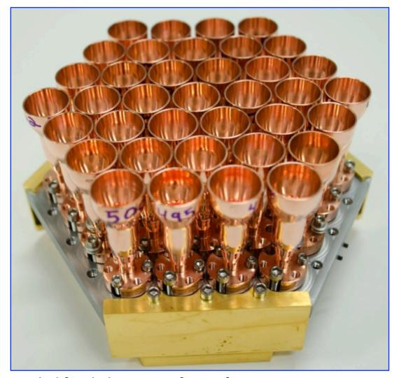
90-GHz feedhorn-coupled focal plane array for performing Cosmic Microwave Background (CMB) measurements
