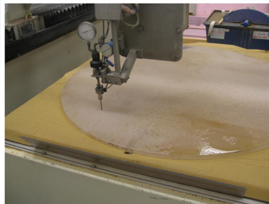
Rounding the glass face plate
