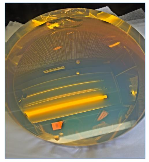
Primary mirror for prototype Laser Interferometer Space Antenna (LISA) telescope
