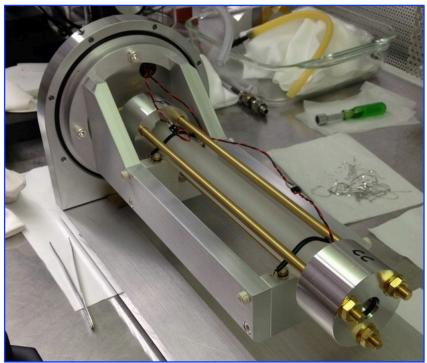
Multi-pressure Brewster cell with removable windows (left) and Immersed cell incorporating piezo actuators (right)
