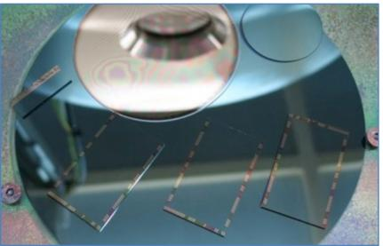
Multi-layer anti-reflection coatings for the FIREBall balloon payload's Electron-Multiplied CCD (EMCCD) detectors; images show wafers before (left) and after (right) Atomic-Layer-Deposition (ALD) coating
