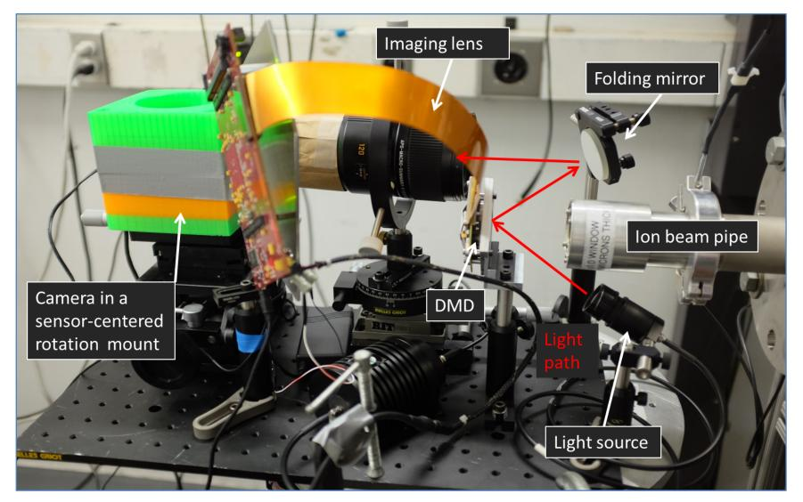
Radiation test setup for Digital Micro-mirror Device (DMD)
