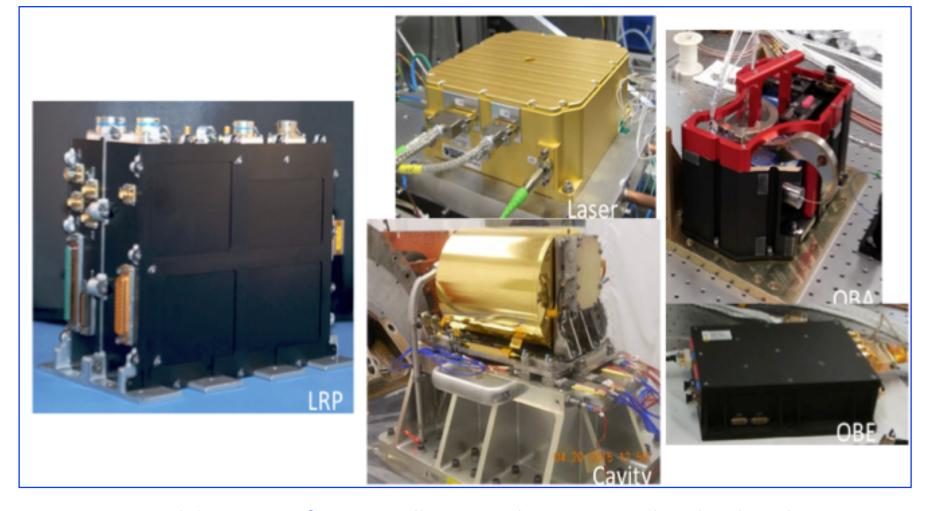
Engineering Model versions of GRACE Follow-On subsystems used to develop phasemeter for the Laser Interferometer Space Antenna (LISA) gravitational-wave (GW) observatory
