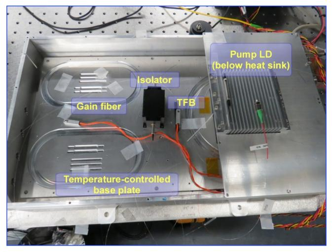
Fiber amplifier for lasers enabling the Laser Interferometer Space Antenna (LISA) gravitational-wave observatory
