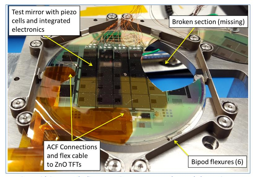
Test X-ray mirror with integrated adjustment piezo actuators and control electronics
