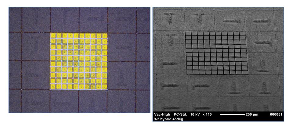
Photo and Scanning Electron Microscope (SEM) image of two types of absorbers for hybrid Transition-Edge-Sensor (TES) arrays fabricated on single Si substrate
