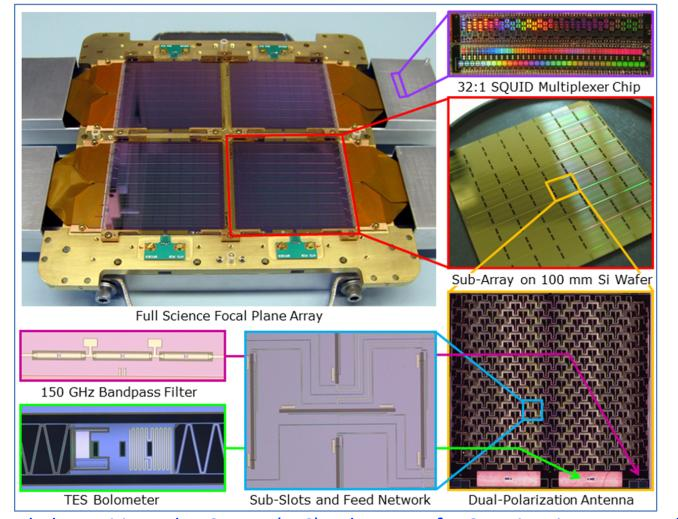
Antenna-coupled Transition-Edge-Sensor (TES) Bolometers for Cosmic Microwave Background (CMB) Polarimetry; lithographed 'Polarimeter on a Chip' Enables Large Arrays
