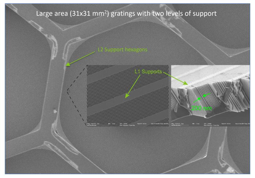
Detail of hierarchical support levels of X-ray Critical-Angle Transmission (CAT) gratings
