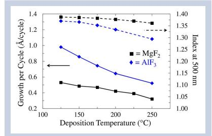
*Fig.* 13. Refractive index and growth per cycle for ALD MgF<sub>2</sub> and AlF<sub>3</sub> deposited on HF-cleaned silicon substrates as characterized by spectroscopic ellipsometry.
