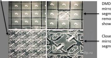
DMD with one mirror segment removed showing driver
