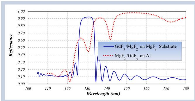
Fig. 9. Reflector design using dielectric stacks of GdF<sub>3</sub>/MgF<sub>2</sub> layer pairs on MgF<sub>2</sub> substrate (blue trace) or Al substrate (red trace).
