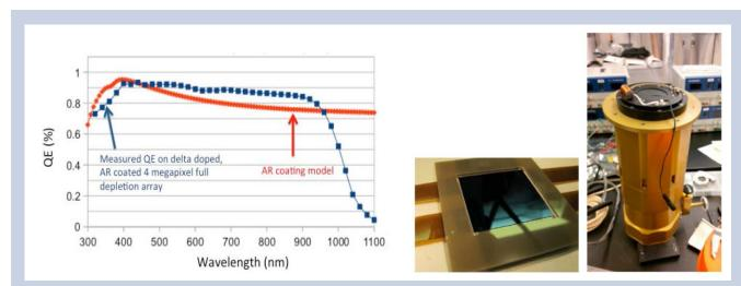
Fig. 4. QE of a broadband AR-coated, delta-doped 12-megapixel p-channel CCD (designed at LBNL and fabricated at Dalsa).
