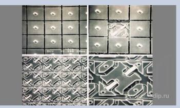
*Fig.* **1.** Clockwise from top left: *DMD; DMD with one mirror segment removed, exposing driver; close-up of a single mirror segment's driver; and DMD with all mirror segments removed.*
