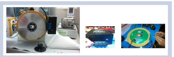
Fig. 3. The Caltech dewar and characterization setup for low-noise measurements expected to fly on FIREBall.
