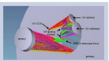
*Fig. 2. Example of UV MOS optical design, showing possible location of DMD.*
