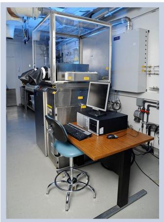
**Fig 11.** ALD coating system at JPL; gas feed-throughs and process controls enable AIF<sub>3</sub> and MgF<sub>2</sub> coatings development.
