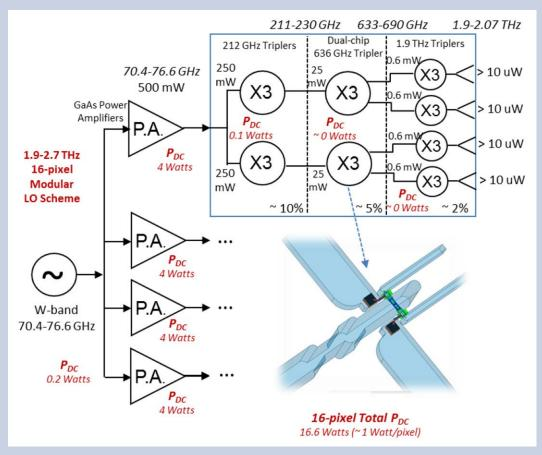
Fig. 3. A modular LO system allows for a compact 16-pixel array receiver.
