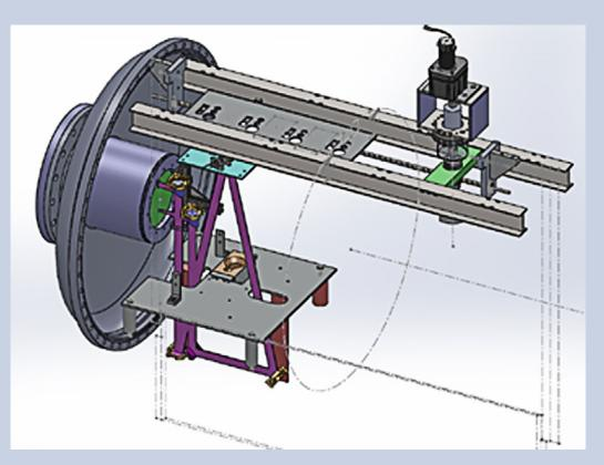
*Fig. 2.* Upgrades to the coating chamber fitted with FUV optical monitoring system and sample transport and masking mechanism to enable multiple coatings without breaking vacuum (courtesy: Zecoat Corp.).
