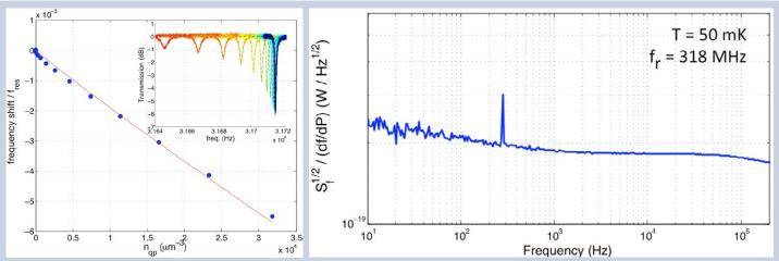
*Fig. 3.* Left: Calibration of detector sensitivity using thermal measurements. The resonance frequency is measured vs. bath temperature (inset). The response of the detector to absorbed power is inferred from the measured frequency shift vs. thermal quasi-particle density. Right: Measured frequency noise spectrum expressed in NEP units using the thermal response data and assuming a quasi-particle lifetime of 1 ms.
