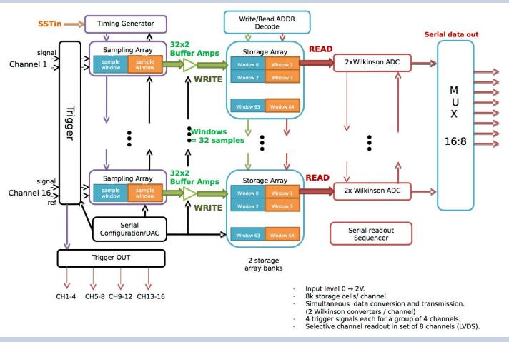
Fig. 3. Functional schematic of the HalfGRAPH2 ASIC design (described in detail in the text).
