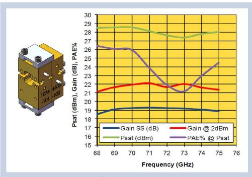
**Fig. 4.** A commercially-available MMIC amplifier will be packaged in a waveguide block for insertion into the LO system. The curves show the expected gain, saturated power, and power-added efficiency (PAE) performance as a function of frequency.
