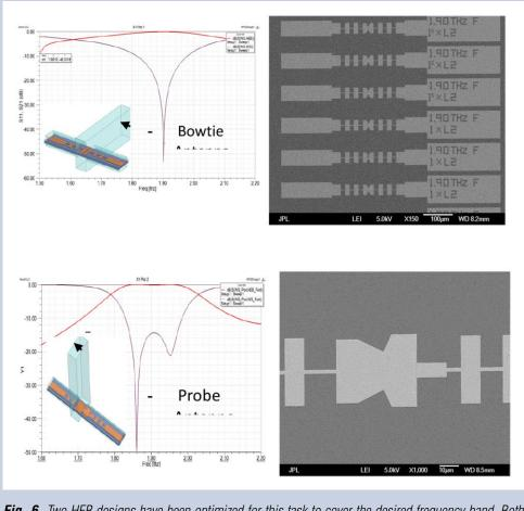
**Fig. 6.** Two HEB designs have been optimized for this task to cover the desired frequency band. Both offer good performance over the required frequency range to cover [CII] and [OI] fine structure lines. These chips are currently being fabricated.
