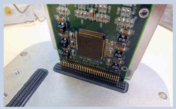
*Fig. 5.* External side of detector showing 80 contact feed-throughs (×2) sealed with epoxy and a 64-channel preamp board plugged into one axis.
