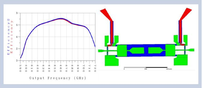
*Fig. 5.* An optimized second-stage tripler will provide sufficient power to pump the final-stage tripler, which will produce the 1.9 THz power required to pump the HEB mixers.
