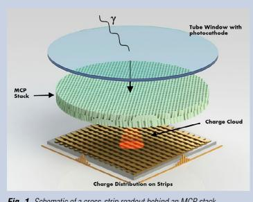
Fig. 1. Schematic of a cross-strip readout behind an MCP stack.
