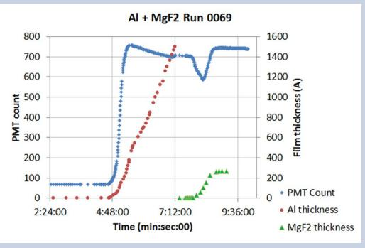
Fig. 5. FUV monitor diagnostic signal while growing AI film followed by MgF<sub>2</sub> film.
