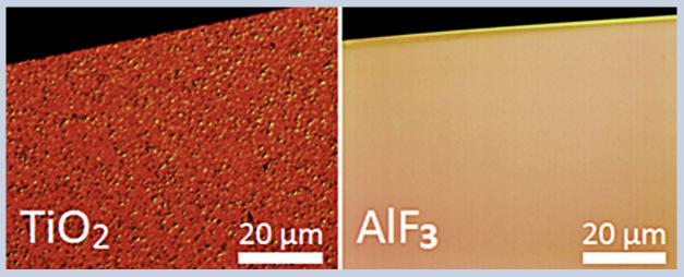
*Fig. 12.* Optical interference micrographs of 100 nm  $TiO_2$  deposited by ALD on silicon at 250°C showing significant grain structure, compared to a 100 nm AIF<sub>3</sub> deposited by ALD at 200°C imaged under similar conditions.
