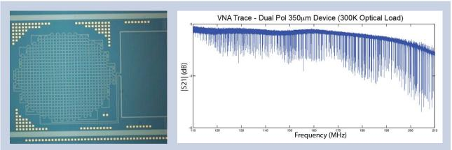
**Fig. 1.** Left: Micrograph of single detector (TiN KID) in an array that will be tested on the CSO telescope in August 2014. The square grid with circular boundary at left is the photosensitive inductive element of the KID with a 540-µm diameter, appropriate for a micro-lens-coupled device operating at 350 µm. Right: Vector Network Analyzer "sweep" of frequency range occupied by the KIDs, showing absorbed power at the resonance of each of the ~500 detectors.
