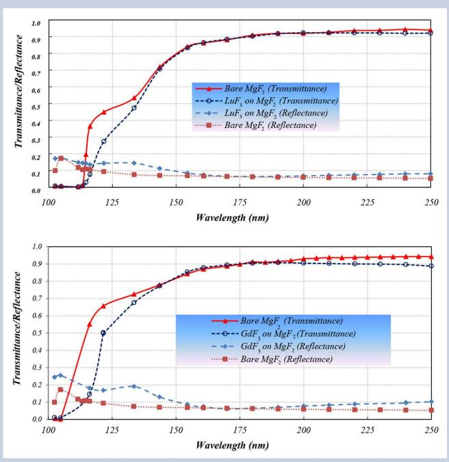
*Fig. 6.* Transmittance and reflectance for LuF<sub>3</sub> (top) and GdF<sub>3</sub> (bottom) films along with data for their respective substrates (MgF<sub>2</sub>).
