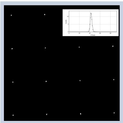
**Fig. 6.** UV image of pinhole mask of 10 µm holes on 1 mm square grid. Inset shows the PSF of a single hole with resolution of ~4 pixels FWHM (20µm).
