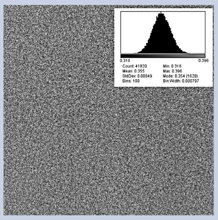
*Fig. 9.* Same image as Fig 8, but divided by deeper flat field. Residual variation is consistent with the expected Poisson counting statistics (2% standard deviation, inset).
