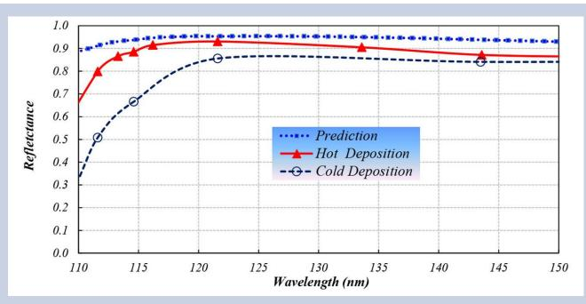
Fig. 3. Predicted and measured FUV reflectance of AI+MgF<sub>2</sub> where MgF<sub>2</sub> was deposited at cold (ambient) and elevated (220°C) temperatures.
