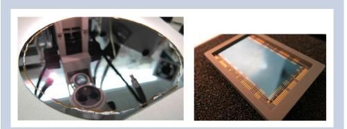
**Fig. 2.** The first 2-megapixel arrays have been processed. QE measured on this device is not absolute but suggested lower than expected values. As a mitigating step, all process steps including MBE (for delta doping) were reevaluated, and possible contamination sources were removed. The next wafers are in various processing steps. One is entirely prepared for delta doping.
