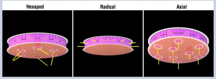
Fig. 4. Different support types demonstrated by mirror modeler.
