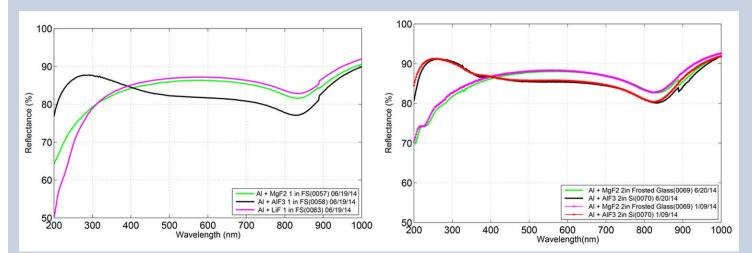
*Fig. 6.* Reflectance measurements in the 200-1000 nm range for single-layer-protected AI mirror samples Left: Measurements for samples on fused silica substrates after about eight months from date of fabrication. Right: Measurements for samples on frosted glass and Si substrates, carried out six months apart. See Table 1 for process details.
