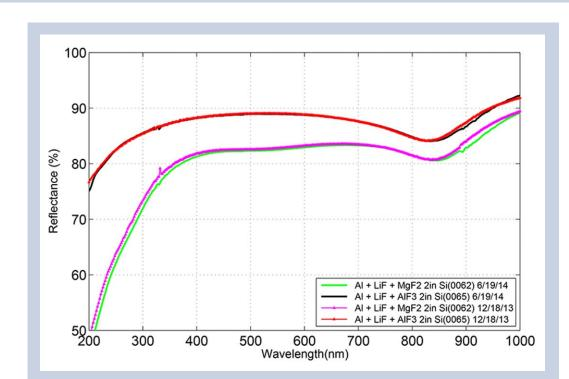
**Fig. 7.** Reflectivity of Al+LiF mirror samples with  $MgF_2$  and  $AlF_3$  protective layers. Measured after six months, these samples, stored in dry nitrogen flow box except during measurements involving a few days of exposure to normal lab environment with ~30-40% humidity, show little degradation. Detailed environmental tests will be conducted soon to check their robustness. See Table 1 for process details.
