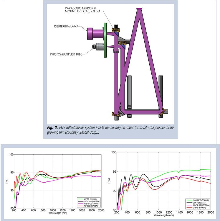
*Fig. 4.* Transmittance spectra of single-layer coatings on UV-grade fused silica substrates (uncoated back side). The numbers in parentheses indicate thickness in Angstroms. Angle of incidence 0°. Left: Coatings of AIF<sub>3</sub>, MgF<sub>2</sub>, and LiF. Right: Coatings of GdF<sub>3</sub>, MgF<sub>2</sub>, LaF<sub>3</sub>, and Na<sub>3</sub>AIF<sub>6</sub>.
