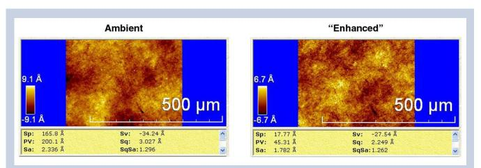
*Fig. 4.* Comparative study of micro-roughness of Al+MgF<sub>2</sub> mirror coatings.
