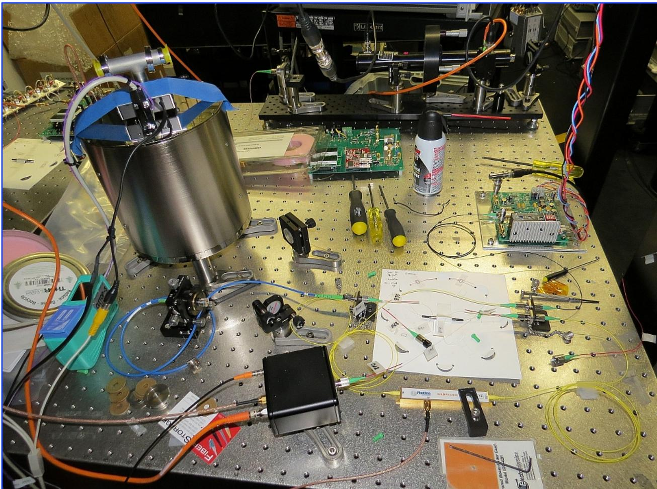
Installation of frequency-reference cavity for oscillator tests used in developing a prototype laser for the Laser Interferometer Space Antenna (LISA) gravitational-wave observatory
