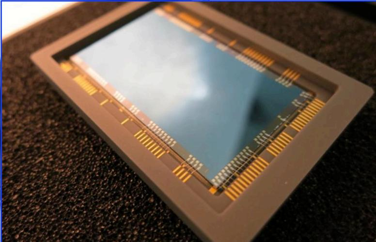
2-Megapixel delta-doped CCD detectors on wafer (left) and as packaged die (right)
