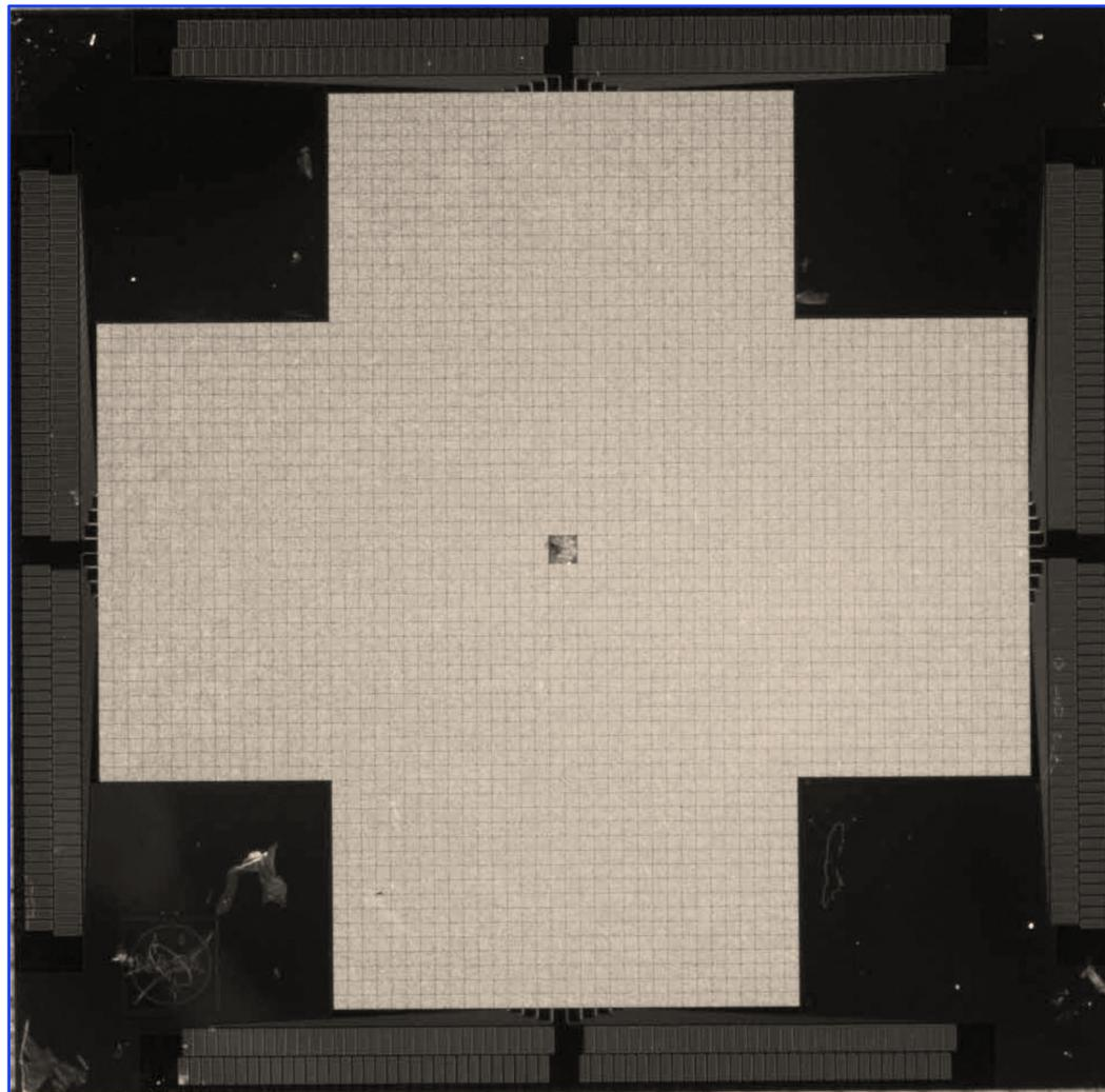
[ATHENA-scale Transition-Edge-Sensor \(TES\) 64×64 array with 16×16-pixel corners removed](#)
