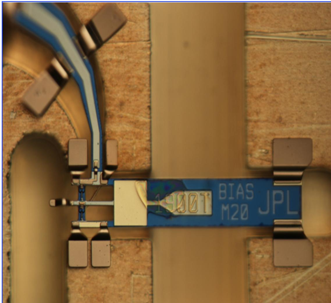
Magnified image of last-stage tripler for controlling pixel power in an array receiver
