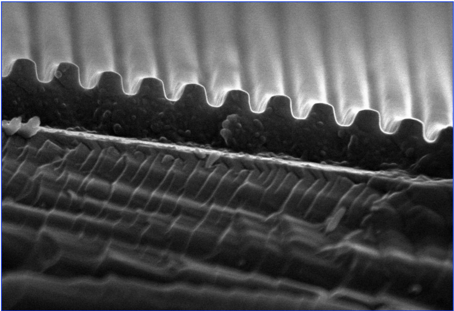
Scanning Electron Microscope (SEM) image of grooved surface for X-ray reflection grating
