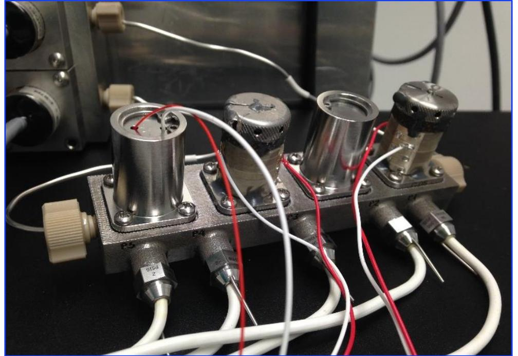
Colloid microthruster propellant tank and controls developed to allow a gravitational-wave (GW) observatory in space
