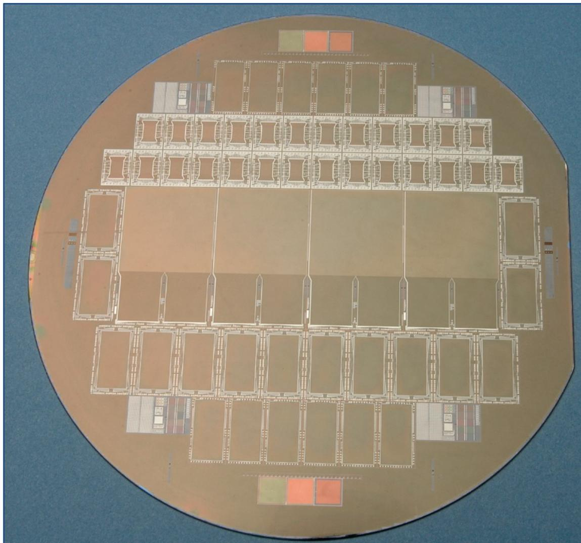
150-mm wafer containing four CCID41 (CCD) X-ray detectors
