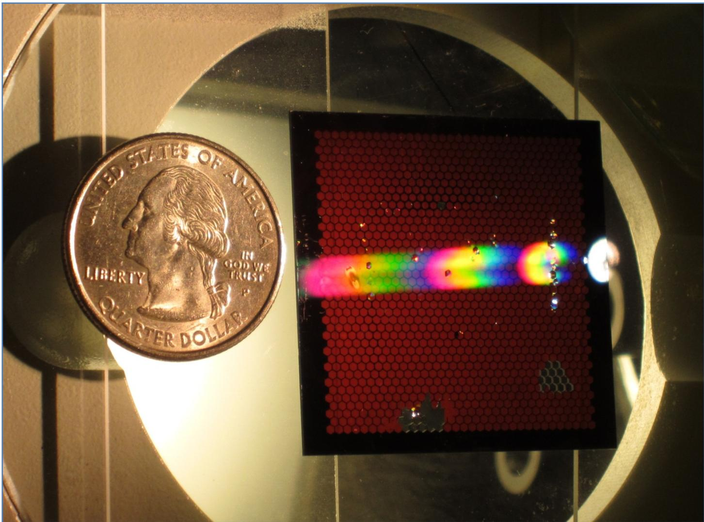
Prototype X-ray Critical-Angle Transmission (CAT) grating with quarter coin for scale
