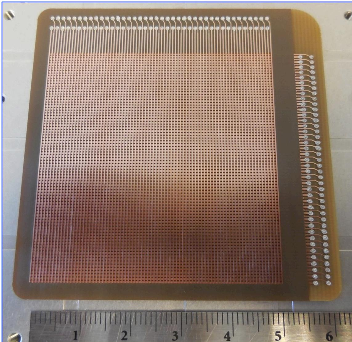
50 mm polyimide cross-strip anode used for 50×50 mm<sup>2</sup> Multi-Channel Plate (MCP) detector
