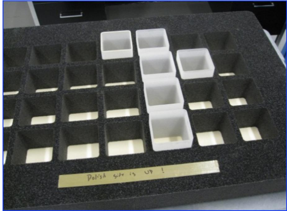
Modulus-of-Rupture (MOR) boxes cut out of glass boule using abrasive water jet (left) and placed in storage fixture (right) for future low-temperature-fusion (LTF) assembly
