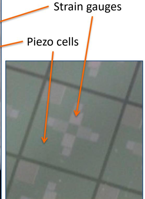
Strain gauges mounted to piezo cells to allow figure adjustment of thin X-ray mirrors
