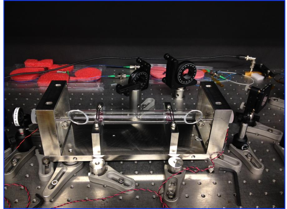
Gas cell test assembly (left) and same cell with Brewster windows (right)
