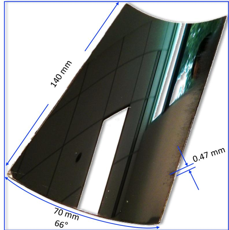
Silicon block with polished cylindrical surface (left) and lightweight silicon X-ray mirror substrate
