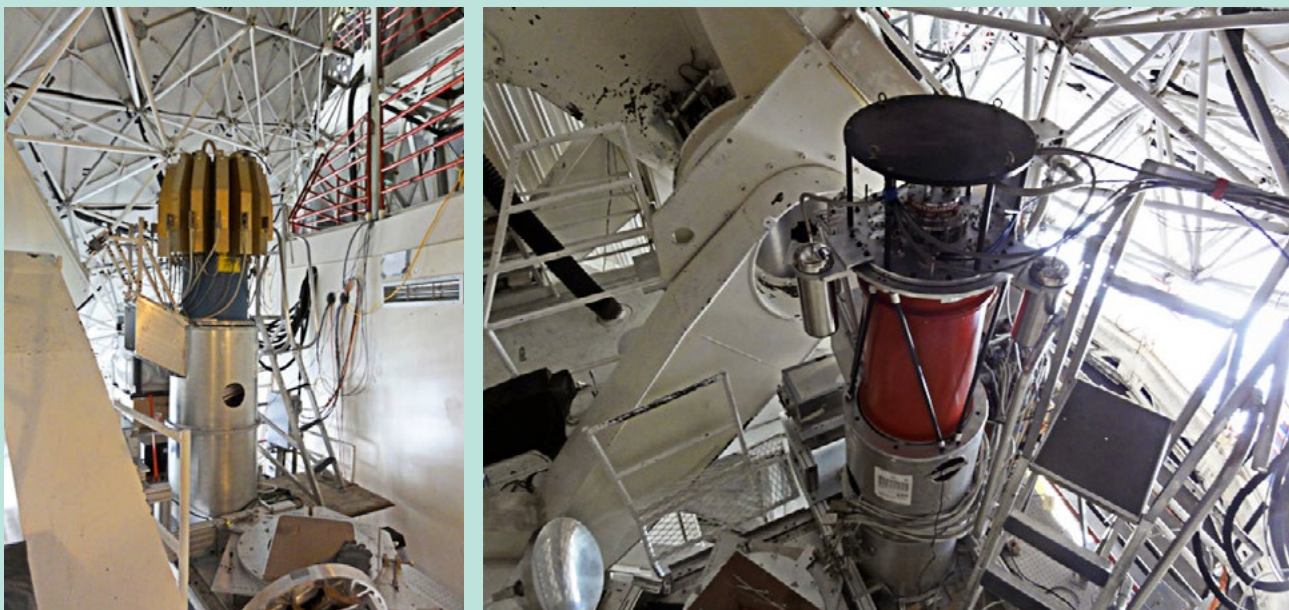
Figure 3. LEFT: The CSO's Submillimeter High Angular Resolution Camera 2 (SHARC-2) 350 \mu\text{m} camera, which contains a (non-multiplexed) 384-pixel micromachined silicon "pop-up" bolometer array. The massive array of preamps and wiring needed for detector array readout is visible on top of the liquid helium cryostat (blue). RIGHT: MAKO, mounted at the SHARC-2 position at the CSO.
