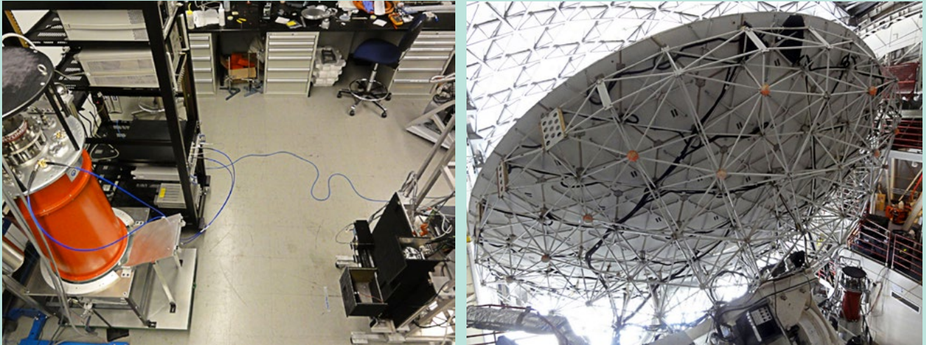
Figure 1. LEFT: The MAKO instrument undergoing laboratory tests at Caltech. The entire 432-pixel array is read out using a pair of RF coaxial cables, colored blue, visible against the cryostat. RIGHT: MAKO at the Caltech Submillimeter Observatory on Mauna Kea, HI. MAKO is visible in the lower right corner.
