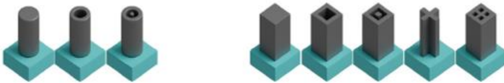
Figure 8. A range of possible nanopost geometries based on round or square symmetry (adapted from ref 37).
