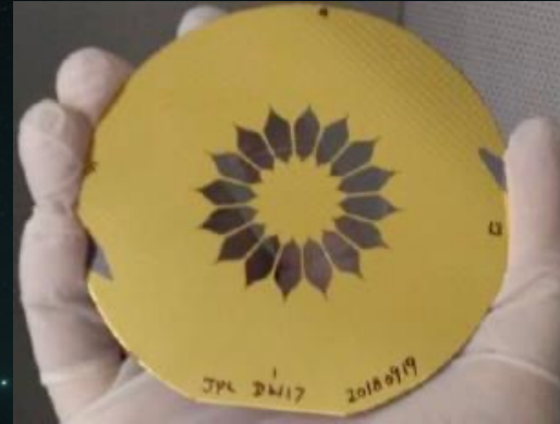
5-cm diameter Starshade etched in silicon
