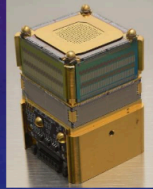
A 244-pixel array of TESs optimized for soft x-ray spectroscopy packaged with microwave SQUID mux readout
