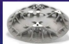
Topology optimized backing structure for a telescope mirror
