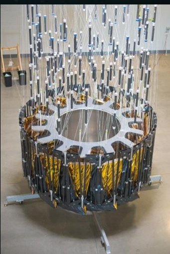
Stowed and partially deployed 10 m disk with optical shield
