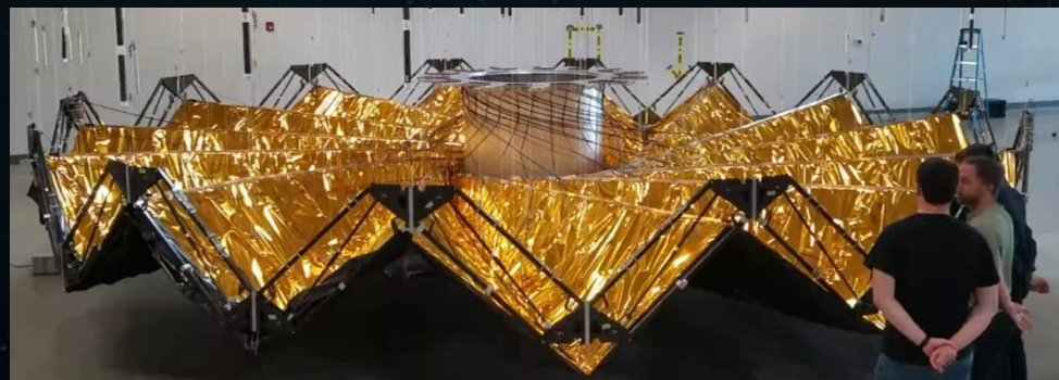
Stowed and partially deployed 10 m disk with optical shield
