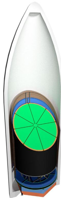
**Figure 2-13:** (left) The *Origins* launch configuration is sized to fit the SLS and BFR launch vehicles. (SLS launch fairing shown).
