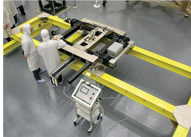
**Figure 2-45:** Variable Center of Gravity Mechanism
