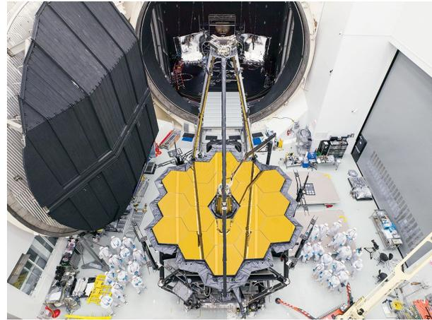
**Figure 2-44:** JSC chamber A supports *Origins* “Test as you fly”. The JWST Optical Telescope Element and Integrated Science Instrument Module (OTIS) is shown rolling into the JSC Chamber A. Chamber A and its helium cooled shroud provides a perfect environment for thermal verification of *Origins* with and without the spacecraft.
